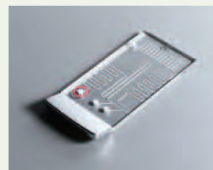
Rapid SNPs Diagnostics System (above) and disposable-type microchip incorporating all processes of DNA extraction, amplification, and detection (below)
