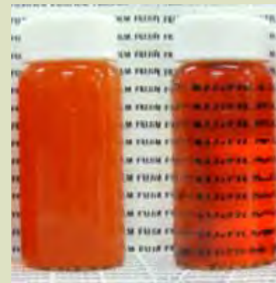
Coarse dispersion liquid (left) and nano-emulsification liquid (right) show differing degrees of permeability.
